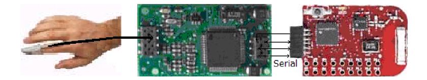
Micro Power Oximeter Board connected to eZ430RF2500
