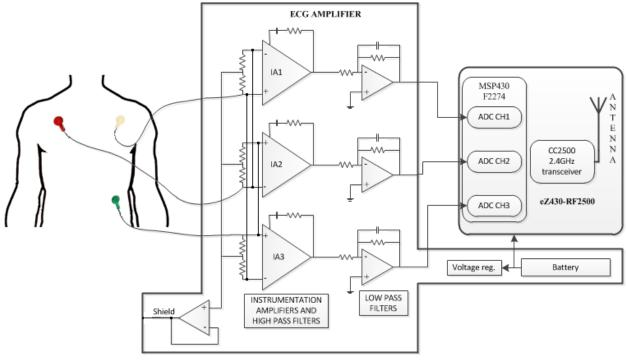
ECG amplifier connected to wireless module
